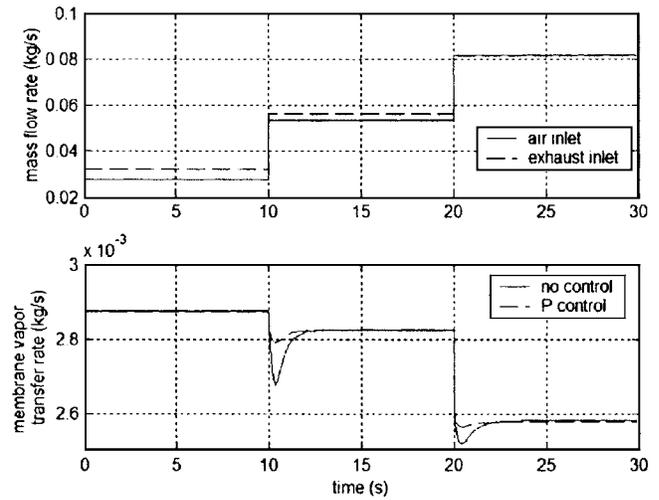
Fig. 14 Membrane vapor transfer rate under two conditions: No control vs  $P$  control
