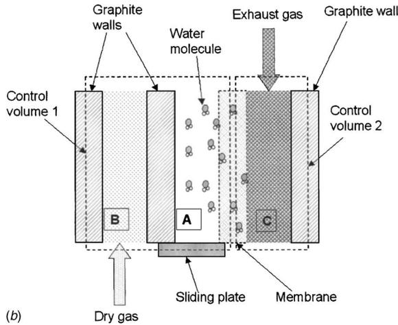
**Fig. 3** (a) Three channels of a humidifier unit: Exhaust gas channel (right), humidification channel (center, open), and heat exchanging channel (left, closed). (b) Three channels of a humidifier unit: Exhaust gas channel (right), humidification channel (center, closed), and heat exchanging channel (left, open).
