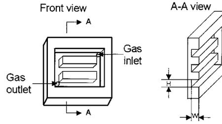
**Fig. 2 Humidifier channel plate**
