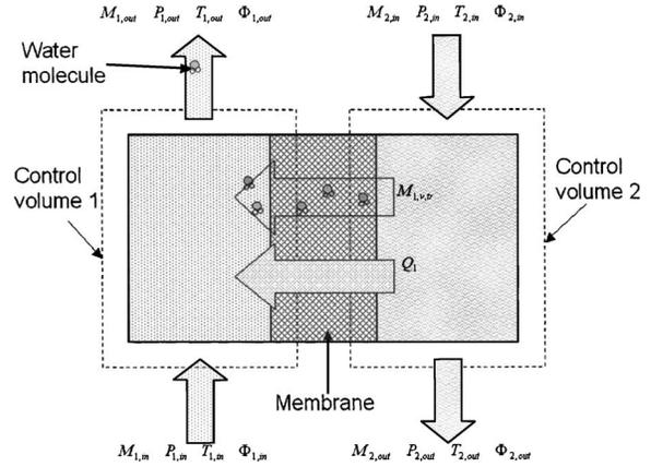
**Fig. 4** Control volumes of one humidifier unit
