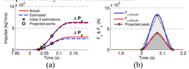
Fig. 11 Comparison of actual and projected impulse and impact forces: (a) Collision impulses, (b) Collision forces
