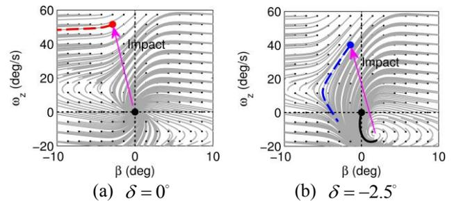
Fig. 7 Vehicle motion on the phase plane with  $v_x = 30$  m/s (Each dot represents an initial condition and each gray line is propagated vehicle motion traces from the dot). An impact, which causes  $\Delta \omega_z = 50^\circ / s$ ,  $\Delta \beta = -3^\circ$ , applied when (a) neutral steering, and (b)  $-2.5^\circ$  steering.
