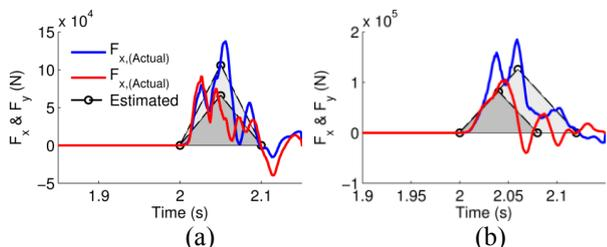
Fig. 13 Comparison with experimental crash data NHTSA crash test no.: (a) v04667, (b) v04955
