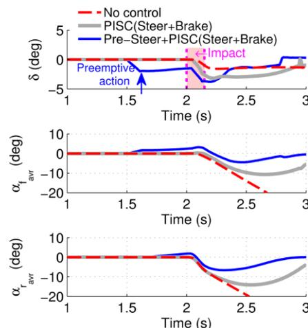
Fig. 17 Tire slip angle comparisons with wheel steering angle actions under an impact condition ( $\alpha_{f_{avr}}, \alpha_{r_{avr}}$  : average slip angles of front two tires and rear two tires)
