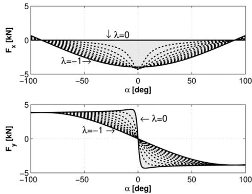
Fig. 3 Tire model showing longitudinal and lateral tire forces (Dotted lines are forces with  $\lambda \in (-1, 0)$ )
