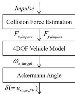
Fig. 9 Feedforward control block structure
