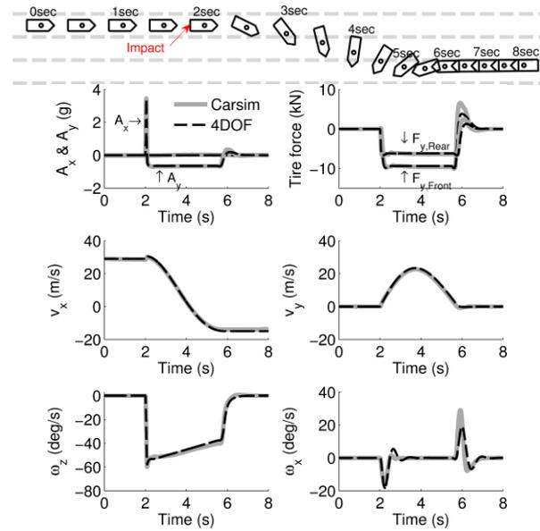
Fig. 10 Vehicle model response validation (No control action is involved. Initial speed:  $v_x = 30$  m/s)
