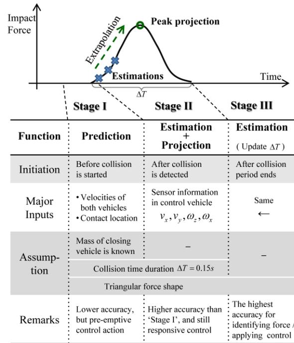
Fig. 4 Function descriptions of the three stages of collision force estimation
