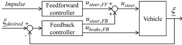
Fig. 8 Block diagram of the control structure,  $\underline{\xi} = [v_y \ \omega_z]^T$
