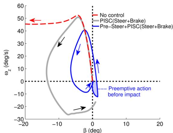
Fig. 18 Evolution of the vehicle motion trajectories on the slip angle-yaw rate phase plane ( $\beta - \omega_z$ ) under an impact condition
