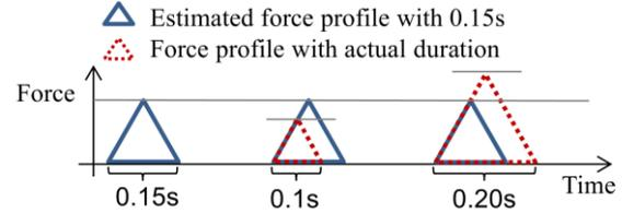
Fig. 6 Force levels with different crash time durations
