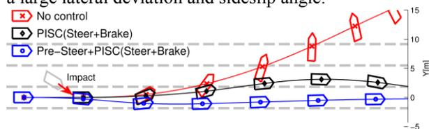
Fig. 15 Trajectories of the vehicles under imposing an impact forces with a vehicle to vehicle collision
