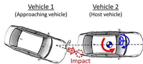
Fig. 1 A crash scenario showing a counter-steering control to negate the vehicle motion due to an impact
