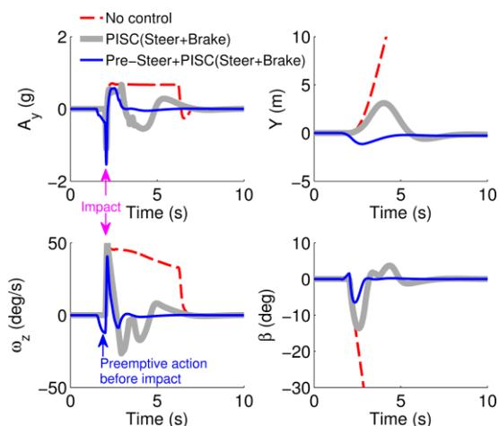
Fig. 16 Test result comparison. (vehicle motion without control, with a steering and brake control during and after the impact (PISC), and with preemptive counter-steering control before the impact )
