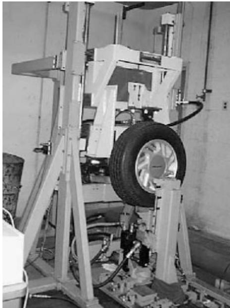
Figure 5. The quarter car active suspension test rig.
